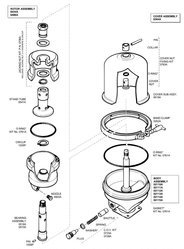
\*SEALS KIT P.N. 0761A COMPRISES OF: C.O.V. WASHER, FILTER BODY O RING, CVR NUT O RING, RTR BODY O RING & BASE GASKET
